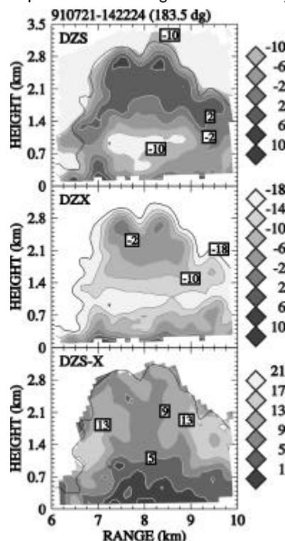
Fig. 1. An example of a developing cumulus cloud, showing a weak mantle echo, flat echo bases at X-band and a weak-echo region near cloud base. (Fig. 12 from (Knight and Miller 1998)).
