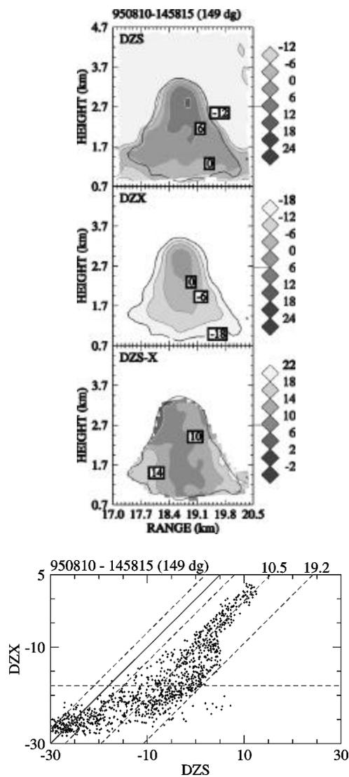
Fig. 2 (a). A developing cumulus cloud, showing a strong correlation between DZS and DZX, and a difference  $DZS-X$  of about 10 dBZ. (b) Scatterplot of DZS versus DZX. (Figs. 10 (c) and 11 (c) from (Knight and Miller 1998)).
