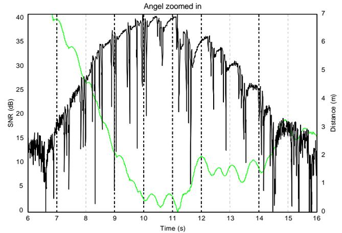
**Figure 5.** Zoom of the Angel in Fig. 3. The highly fluctuating line is the signal-to-noise ratio of the Angel. The smooth grey line is the unwrapped phase of the Angel converted into a measure of the relative distance to the radar.
