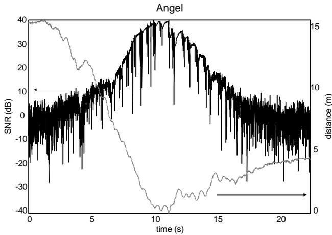
**Figure 4.** Measurement of an Angel with DARR. This line graph is made from a cross section of the Angel in Fig. 2 at 2235 m. The highly fluctuating line is the signal-to-noise ratio of the Angel. The smooth grey line is the unwrapped phase of the Angel converted into a measure of the relative distance to the radar.
