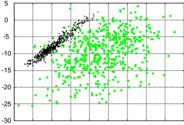
**Figure 2.** Scatter plot of the radar reflectivity factors at X and S-band for part of the mist and downdraft measurement. The crosses are data points taken in the mist and the grey dots are data points taken in the downdraft. The lines represent an equal radar reflectivity factor (pure incoherent Rayleigh scattering) and a 19 dB stronger reflections at S-band (pure coherent scattering with -5/3 slope).
