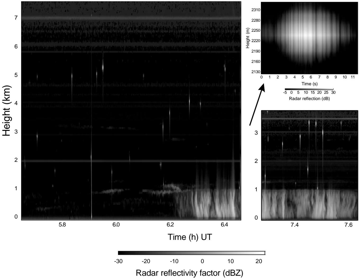
**Figure 3.** Measurement of Angels performed with DARR on the 4th of September 1996. The picture at the left and bottom right show the radar reflectivity factor calculated using the standard processing with a temporal resolution of 5.12 s. The high temporal image (top right) has a resolution of 5 ms. To get local summer time add two hours.
